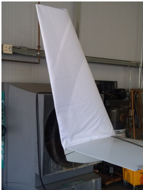
Velocity Vertical Stabilizer Covers, test fit cover
