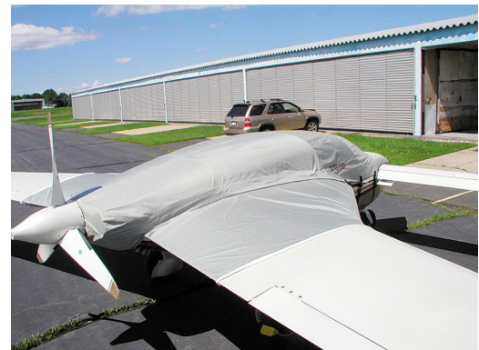
Velocity Canopy/Engine/Nose with Abbreviated Wing Covers
