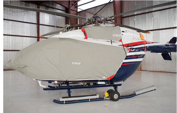
Upper Deck Plugs/Cover, extended to cover aft intake vents Bubble Cover w/ nose mounted radome, Upper Deck Plugs/Cover
