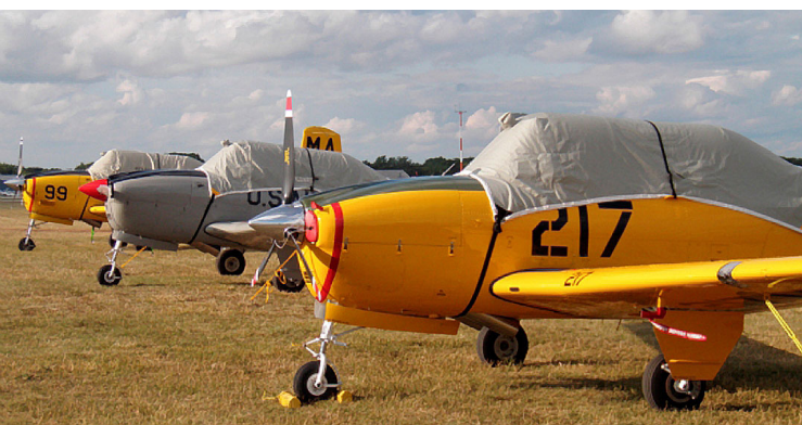
T34 Canopy Covers & Engine Inlet Plugs
