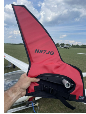
Schempp-Hirth Ventus-2B winglet/wingtip pads
