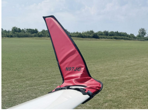
Schempp-Hirth Ventus-2B winglet/wingtip pads
