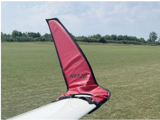
Schempp-Hirth Ventus-2B winglet/wingtip pads
