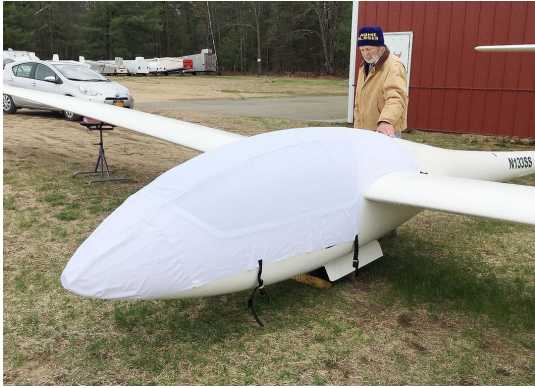
Grob 102 Astir CS Canopy/Nose Cover (test fit)
