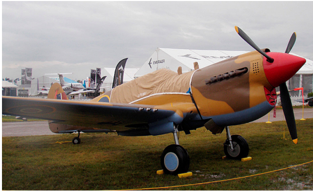
P40 Canopy Cover & Engine Inlet Plugs
