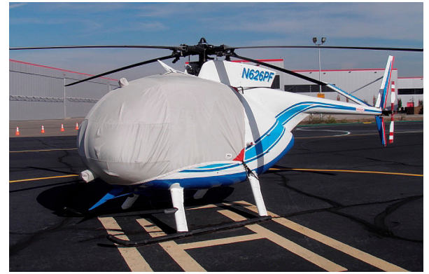
MD500C Bubble Cover with Wire Strike detail
