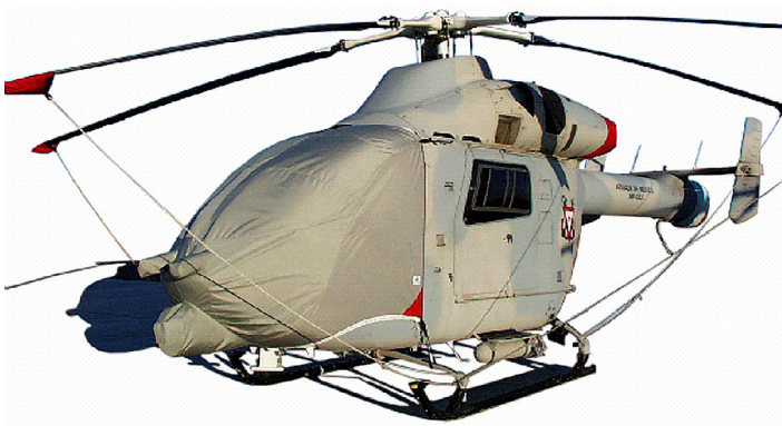
MD900 Forward Bubble Cover (w/Radome), Blade Tie-Downs
