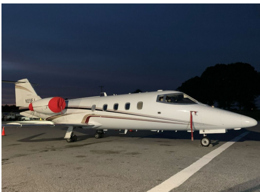
Lear 60 Cockpit Heatshields, Tri-Fold Engine Covers
