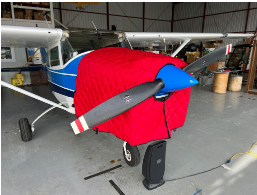
Insulated Hangar Blanket on Cessna 182
