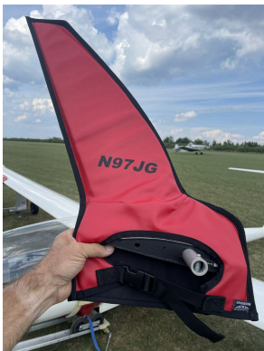
Schempp-Hirth Ventus-2B winglet/wingtip pads
