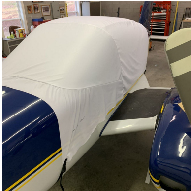
Wing Derringer Canopy Cover, test fit
