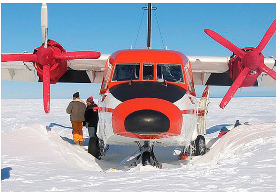
Casa 212 Insulated Engine & Propellor/Spinner Covers
