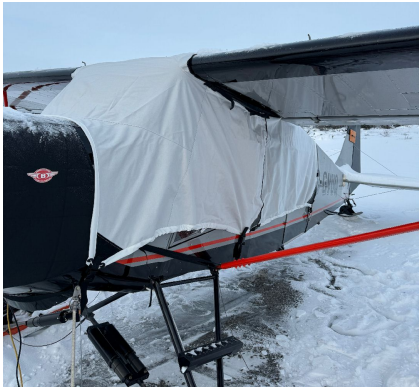
Bushmaster Canopy & Insulated Engine Covers
