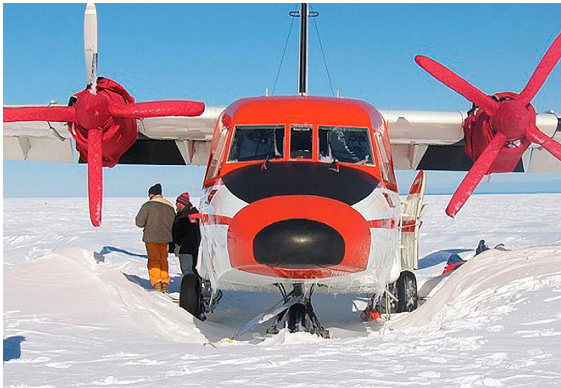
Casa 212 Insulated Engine & Propellor/Spinner Covers
