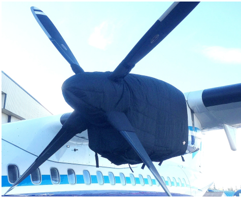
ATR-72-202 Insulated Engine & Prop Hub Covers
