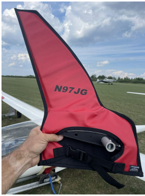
Schempp-Hirth Ventus-2B winglet/wingtip pads
