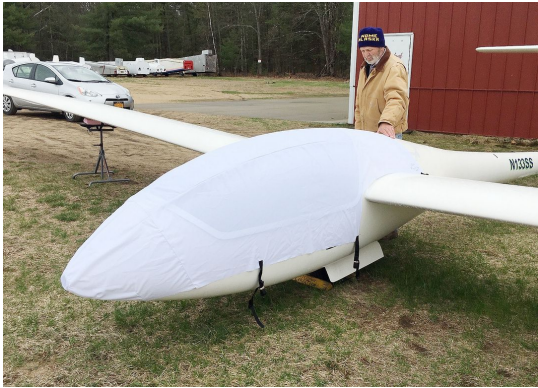
Grob 102 Astir CS Canopy/Nose Cover (test fit)
