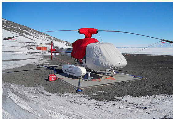
AS350 Bubble Cover w/ Cargo Mirror, Blade Tie-downs, Insulated Engine, Insulated Main Rotor Hub & Insulated Tail Rotor Covers
