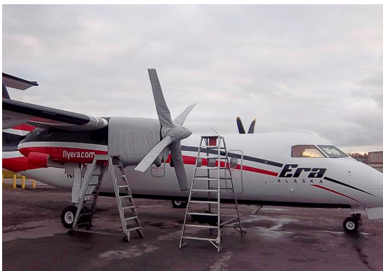
Dash 8 Insulated Engine & Prop Covers
