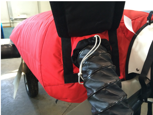
Cessna 402 Insulated Engine Cover with Heater
