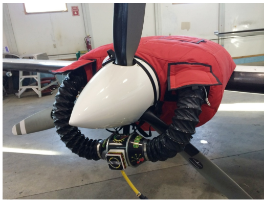
Cessna 402 Insulated Engine Cover with Heater
