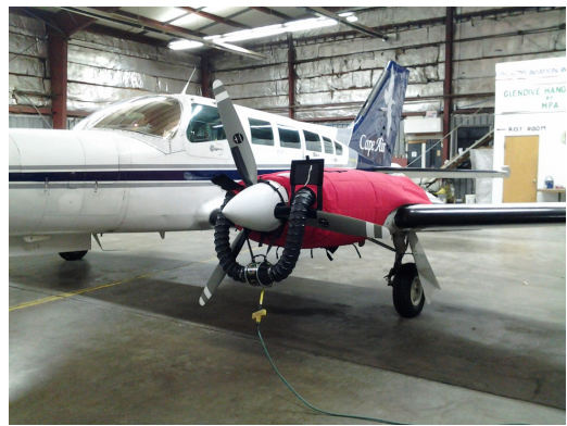
Cessna 402 Insulated Engine Cover with Heater
