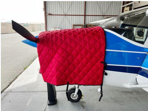
Insulated Hangar Blanket on Cessna 182
